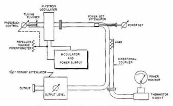
Figure 1. Basic circuit,-hp- 626A/628A.
