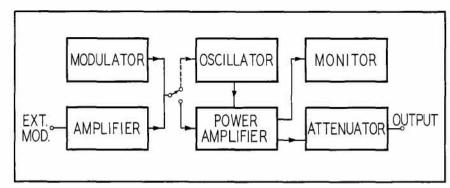
Figure 1. Block diagram of Signal Generators in Group I.
