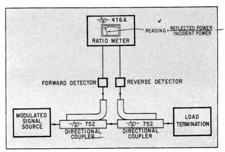
Figure 4. Typical Reflectometer setup.
