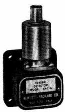
Now available for H, X and P bands, Model 421A is an accurate, square-law detector specifically designed for reflectometer measurements. -hp- H421A covers 7 to 10 KMC; -hp- X421A covers 8.2 to 12.4 KMC; -hp- P421A covers 12.4 to 18.0 KMC. Reflection coefficients as low as 0.01 may be measured with sensitivity of 0.01 v/0.1 mw, maximum SWR of 1.5, and frequency response of ±2 db. The square-law characteristic is within ±1 db from 0 to -40 dbm when operated into
