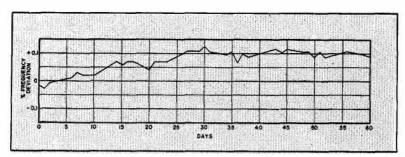
Figure 5. Long-time stability curve of circuit using wire-wound resistors and temperature compensation.
