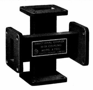
752, a single oscilloscope presentation of SWR vs. frequency is easily made. In this operation, output of the auxiliary arm of the coupler is detected, amplified and applied to the vertical plates of the oscilloscope tube. The frequency applied to the system is swept and a voltage proportional to this frequency is applied to the horizontal plates of the oscilloscope. The resulting trace is a plot of reflection vs. frequency.
