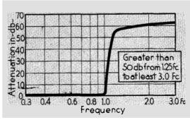
Figure 2. Typical rejection characteristics.
