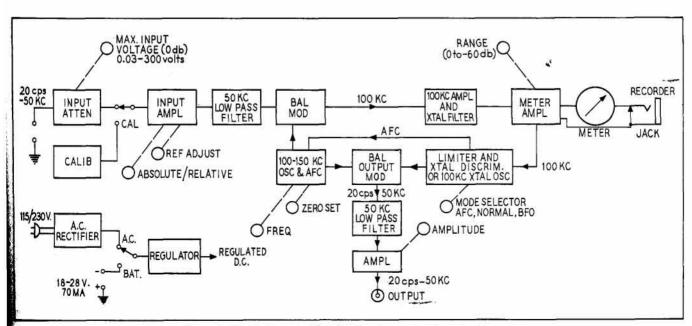
Figure 1. Block diagram, Model 302A Harmonic Wave Analyzer
