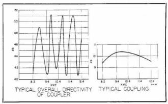
Figure 3. Characteristics, -hp- 752 Coupler - 10 db model.
