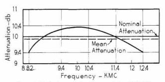
Figure 1. Typical attenuation characteristics, @ X372C 10 db attenuator.
