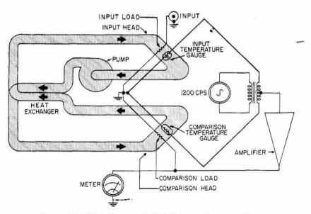
Figure 5. Simplified diagram, @ 434A Calorimetric Power Meter.
