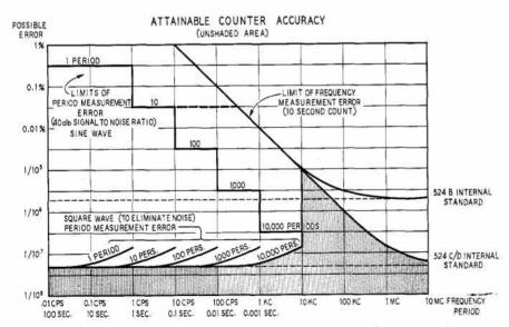
Figure 3. Possible error factor in frequency measurement (@ 524B, 525A).
