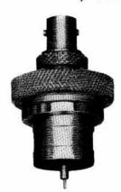
A modified crystal (1N76 or 1N26) plus a small antenna in a convenient housing permitting probe penetration to be varied quickly and easily. Probe position is fixed by a locking ring. Requires no tuning; and sensitivity surpasses most elaborate single and double-tuned probes (particularly between 8 and 18 KMC). Polyiron inserts damp spurious resonances. Frequency coverage 3 to 18 KMC; BNC output jack. For 34" mounting hole as on -hp-809B Carriage (page 144). \$40.00.
