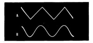
Figure 2. Oscillogram of (A) triangular wave applied to special @ developed shaping circuit and (B) resulting true sine wave.
