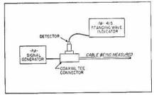
Figure 2. Arrangement of instruments for measuring velocity of propagation.
