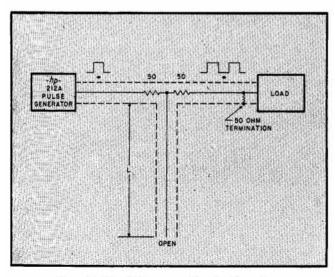
Figure 3. Circuit for generating double pulses.
