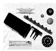
In electronics, special or unusual parts are often hard to find, or prohibitive in cost. To avoid this roadblock to progress, hp- has its own plastics and molding shop, which turns out knobs, escutcheons, Nylon gears, etc.
