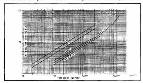
Figure 8. Attenuation vs. frequency curves for several cables.
