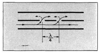
Figure 2. Cross-section, two-aperture coupler.
