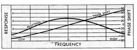
Figure 3. Characteristics of Frequency Determining Network.
