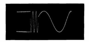
Figure 1. Oscillogram shows freedom from transients as output frequency is rapidly changed.
