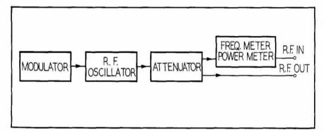
Figure 3. Block diagram of Signal Generators in Group III.
