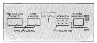
Figure 1. Circuit arrangement, Model 206A.
