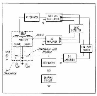
Figure 1. Basic arrangement of instrument circuitry.
