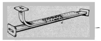
Figure 1. Construction, -hp- 752 Directional Couplers.
