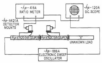
Figure 1. Typical Reflectometer Setup. Note use of two directional couplers back-to-back, with individual detectors, for simultaneous evaluation of incident and reflected powers.
