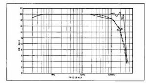
Figure 2. Typical response of 460A Amplifier working into (B) resistive load and (A) using -hp- 410B Vacuum Tube Voltmeter.
