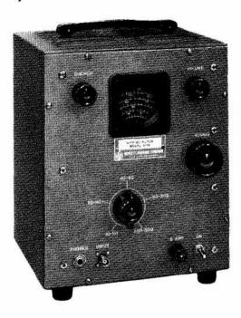
This -hp- instrument is a super-regenerative (AM) receiver covering all frequencies between 10 and 500 MC in 5 bands. It is designed for use with the -hp- 803A Bridge. It offers a high sensitivity of approximately 5 microvolts over the entire frequency band. It is designed for fast, simple operation, and has a single, convenient frequency control directly calibrated in megacycles.
