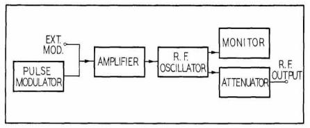
Figure 2. Block diagram of Signal Generators in Group II.
