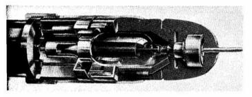
Figure 1. Construction details of @ diode probe.
