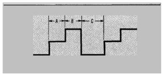
Figure 1. Threshold feature for time interval measurements permits measurement of duration of each step of voltage.
