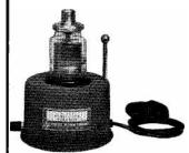
For -hp- 400 series and 410B. Safely measures power voltages to 25 kv. Accuracy  $\pm 3\%$ . Division ratio 1000:1. Input capacity 15  $\mu\mu$ f  $\pm 1$ . Maximum voltage ratings at 60 cps, 25 kv; 100 KC, 22 kv; 1 MC, 20 kv; 10 MC, 15 kv; 20 MC, 7 kv. Usable for dielectric heating, power and supersonic voltages. Price, \$125.00.
