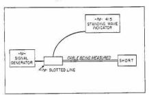
Figure 1. Suggested instrument arrangement for measuring small values of cable attenuation. Unknown cable is placed between slotted line and short.
