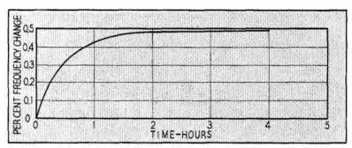
Figure 6. Typical short-term stability of RC oscillator.
