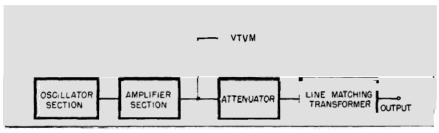
Figure 1. Elements of a signal generator.
