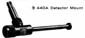
A simple, easily used instrument for detecting rf energy in coaxial or waveguide systems. In coaxial use, covers all frequencies 2.4 to 12.4 KMC. Uses either 1N21 or 1N23 silicon crystal, 1/100 amp. instrument fuse or Sperry 821 barretter. Simple single stub tuning. Type N rf input connector, BNC output jack. With -hp- 442B (below) becomes sensitive, easily tuned detector for slotted waveguide sections. (Detector element not furnished as a part of instrument.) \$85.00.
