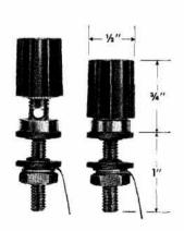
Designed by -hp-, these posts insure a positive connection that can be changed quickly and easily. The recess for "banana" plugs is in the main body of the post to eliminate excessive contact resistance. The cross-hole for permanent connection may be used even when a plug is inserted. The posts have a nylon insulated ferrule. AC-10C (black), \$.30; AC-10D (red), \$.30.
