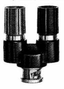
This new -hp- adapter mates with a BNC receptacle, providing an easy method of connecting clip leads, banana plugs or wires to instruments having BNC receptables. The nylon ferrule of the center conductor binding post is colored red; the other ferrule is black. Spacing between the banana plug is 3/4". \$5.00 each.
