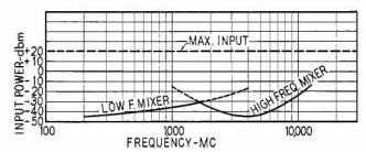
Figure 2. Typical sensitivity, model \$\theta\$ 540B.
