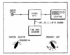
Figure 1. Frequency measurement circuitry in \$\oplus\$ electronic counters (\$\oplus\$ 524 illustrated).
