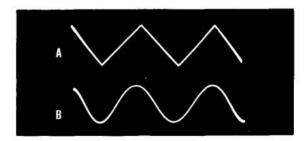
Figure 2. Oscillogram of (A) triangular wave applied to special @ developed shaping circuit and (B) resulting true sine wave.
