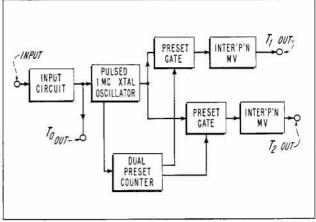
Figure 3. Basic circuit arrangement of -hp-218AR Digital Delay Generator.
