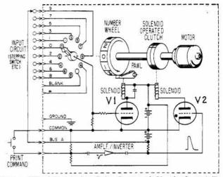
Figure 1. Wheel-Positioning, Print Command Circuit, @ 561A/B.
