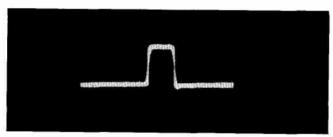
Figure 2. Typical rf pulse envelope, 0.25 µsec, 624C.
