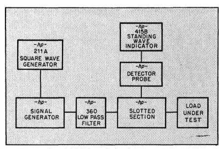
Figure 1. Typical setup for impedance measurements.
