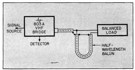
Figure 6. Measurement setup using balun with balanced load.
