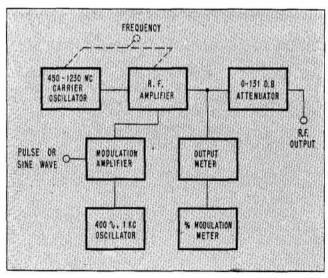
Figure 1. Block diagram, -hp- 612A Signal Generator.
