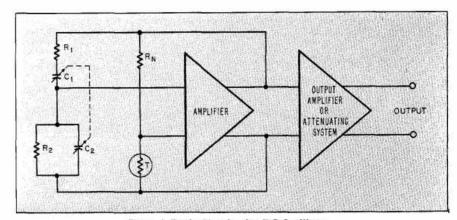
Figure I. Basic Circuit, -hp-RC Oscillator.
